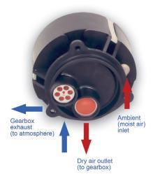
When ambient pressure exceeds gearbox pressure, moisture laden air is drawn into the breather cartridge. After cycling through the desiccant maze, the dried air is delivered to the gearbox.
