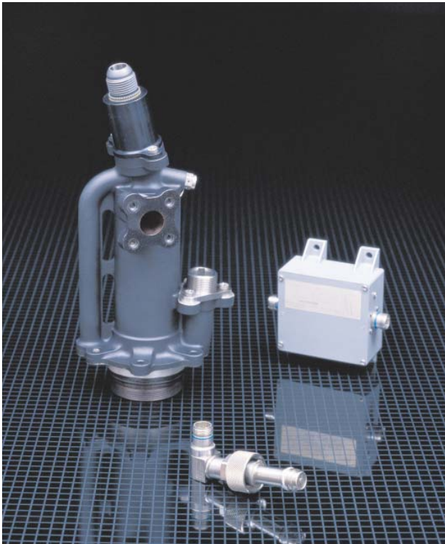
The heart of the system is a magnetic, inductive particle sensor. It captures and retains ferromagnetic debris particles and provides an output signal for each capture.
