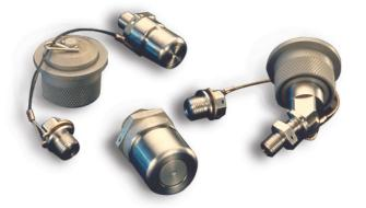
These high reliability units serve a specialized need to allow spillproof, quick-connect oil or hydraulic servicing of aircraft engines, transmissions, generators, auxiliary power units and other aircraft systems. They meet MIL-A-25676 requirements and are available in MS24476-1 and -2 sizes that mate with MS24475-1 and -2 servicing nozzles respectively.
